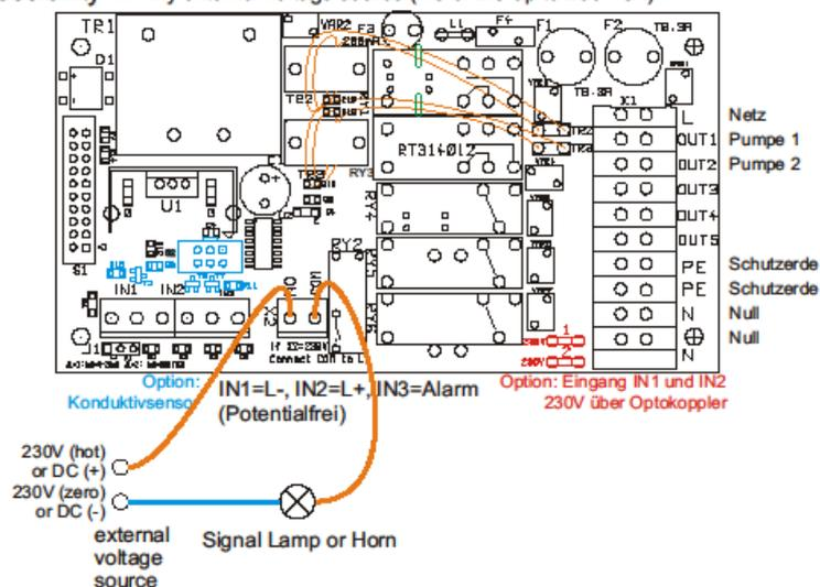
Possibility 1: Internal 230 voltage source (up to 250V 3A)
