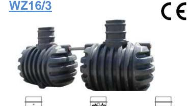
Installation in sand Volume 3 x 3.300 liter Number of PE Van 12 tot 16 2.390 mm Length Width 1.610 mm Height 2.210 mm Height in 1.500 mm Height out 1.450 mm Diameter in/out 110 mm **Diameter manholes** 600 mm Weight 620 kg Flow rate air pump 100 l/min Aeration regime Continuously Consumption/year/person +/- 85 Kw Price – B01 € 8.571,65
