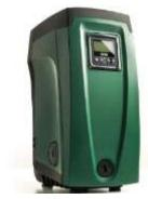
E.sybox is the new integrated system by DAB for water pressure boosting in domestic and residential applications. E.sybox does not require any additional component for its installation because it consists of a self-priming multistage pump, electronics for control and management, pressure and flow sensors, a high-resolution LCD orient able display and an integrated expansion vessel of 2 liters.
